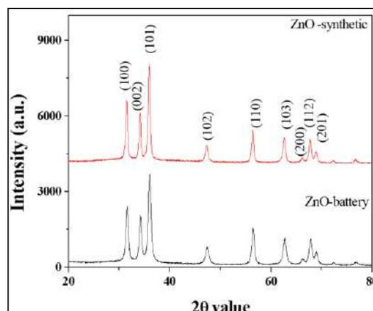
**Fig 1:** P-XRD pattern of ZnO-synthetic and ZnO-battery nanoparticles.
