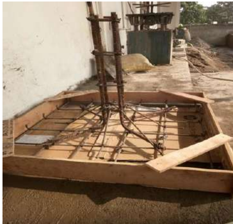
Fig 1: Second specimen, FSW showing the swimmer bars
